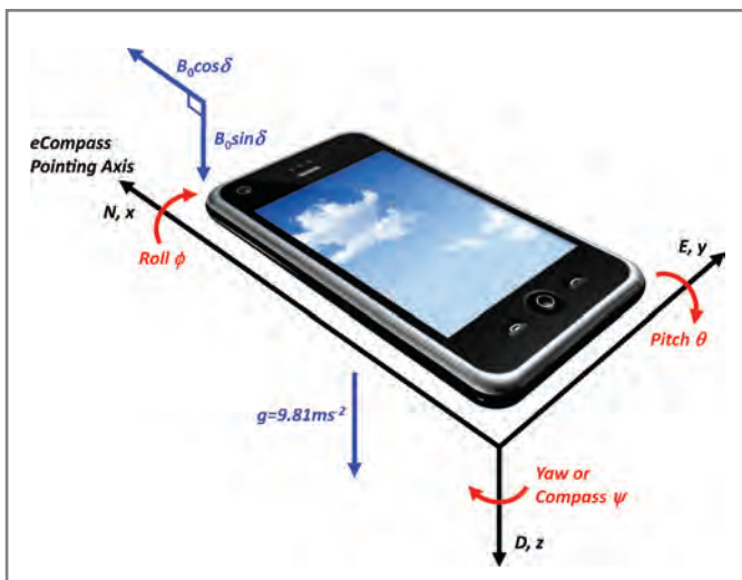
Photo 1—The aerospace north-east-down coordinate system
